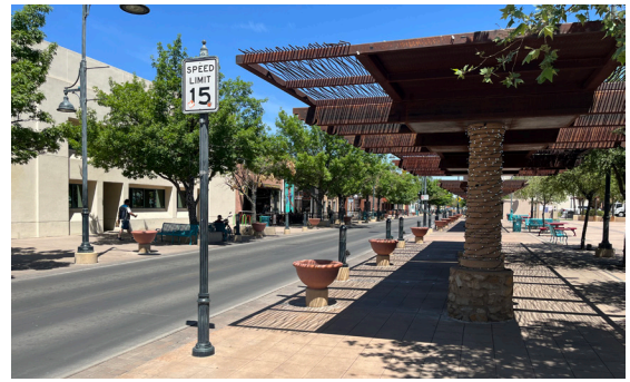
Shade and street furnishings improve comfort and visually narrow the roadway to support slow speeds..
