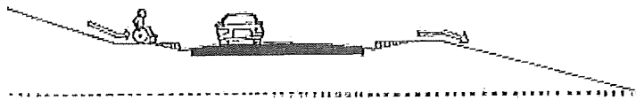
Figure 7-39. GOOD DESIGN: The level area of an intersection should be extended to include the curb ramps and the level landings above them.
